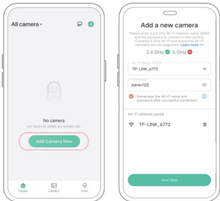
2) To ensure a long distance connection, the camera only supports the 2.4Ghz Wi-Fi with stronger wall penetration capability and does not support Wi-Fi for enterprise level authentication currently. Please ensure that the entered Wi-Fi meets the requirements. After completion, click "Continue" to generate the QR code for pairing the camera.
